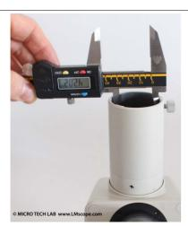
The LM digital adapter has been especially developed for Nikon microscopes with phototubes (42mm internal diameter).
