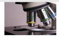
Now swivel in the 10x microscope lens and visually focus the image by means of the microscope focusing mechanism. Plan achromatic, plan fluor or plan apochromatic microscope lenses are optimal for perfect micro images.
